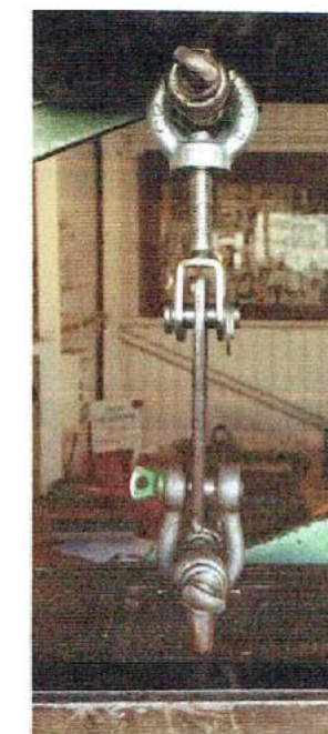
Photograph 1: Fastening arrangement in the first test
